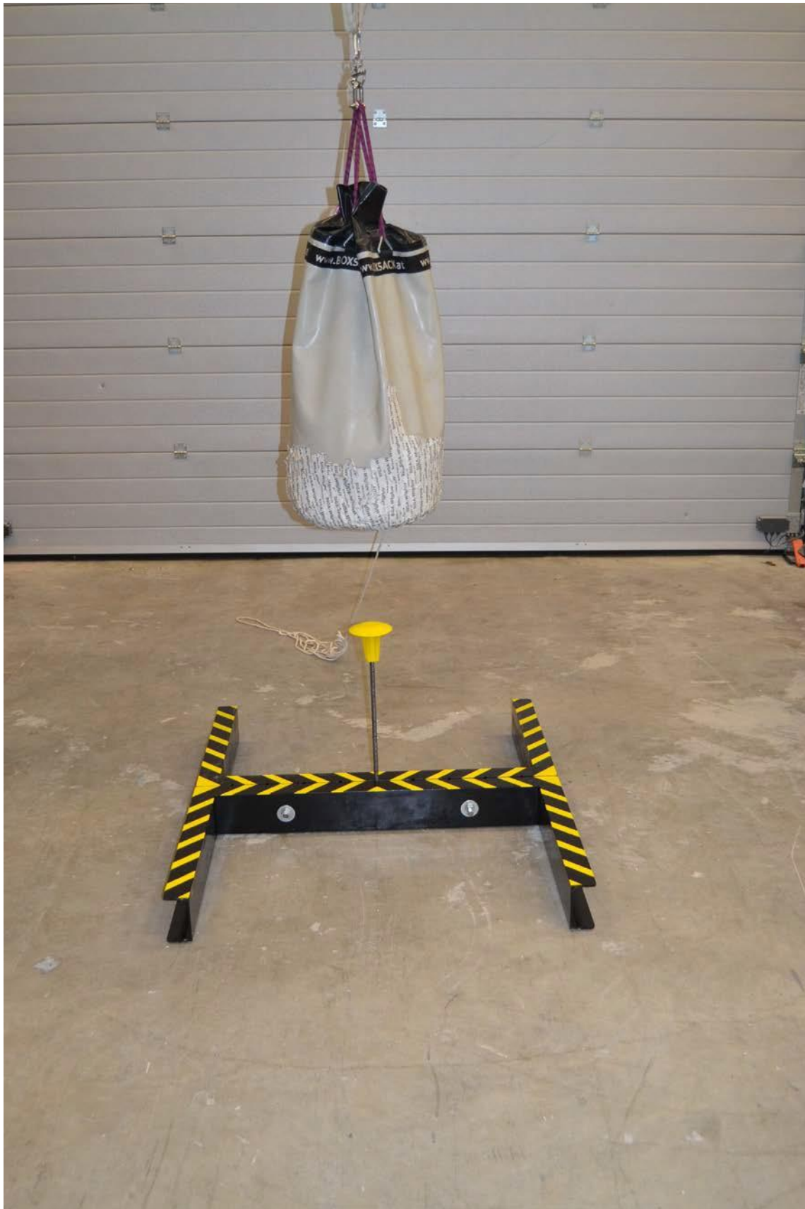
Figure 6: Clamped single rod d=12\text{mm} with centred fall sack
