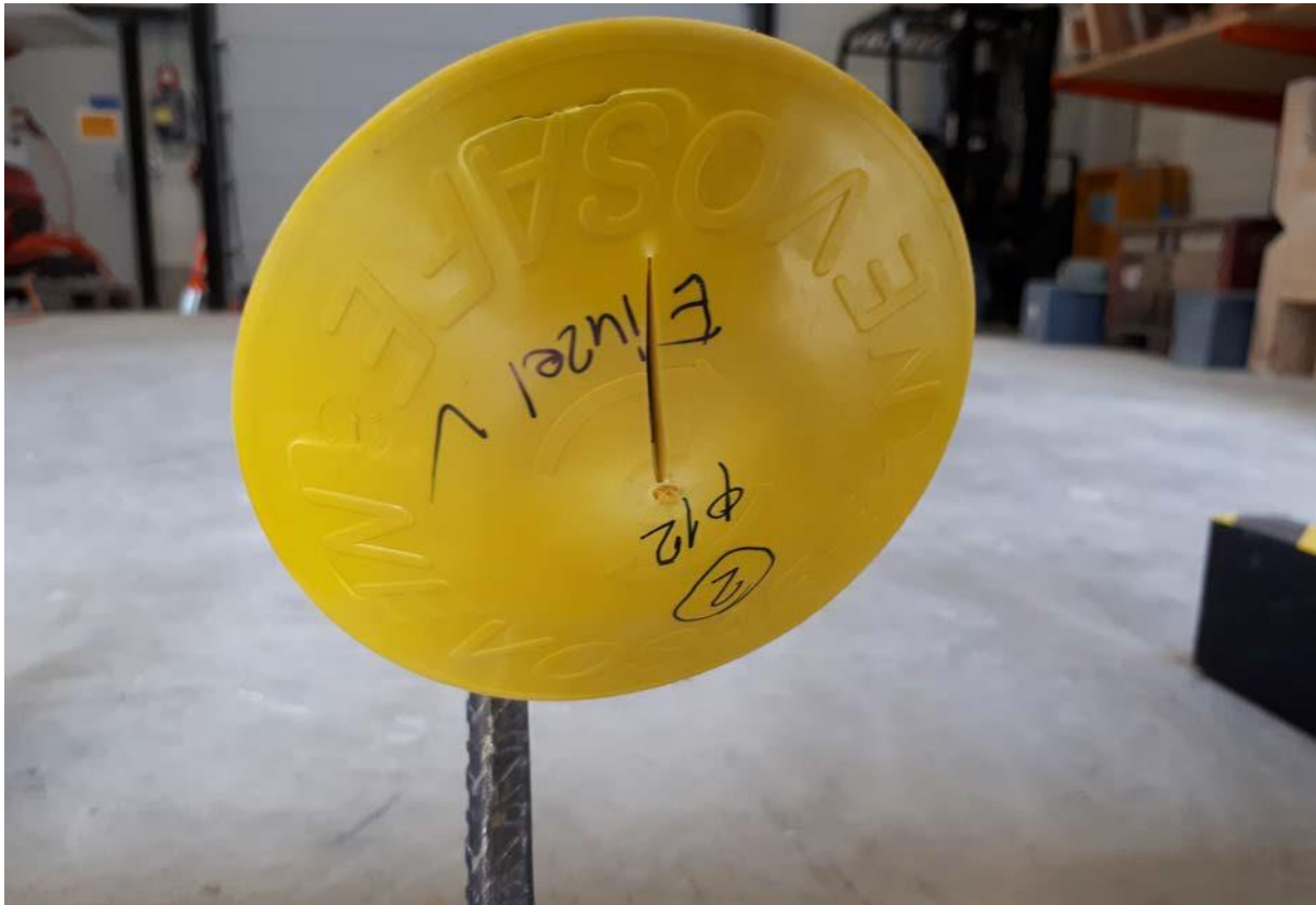
Figure 9: Test body 2 with buckling but without shear punching
