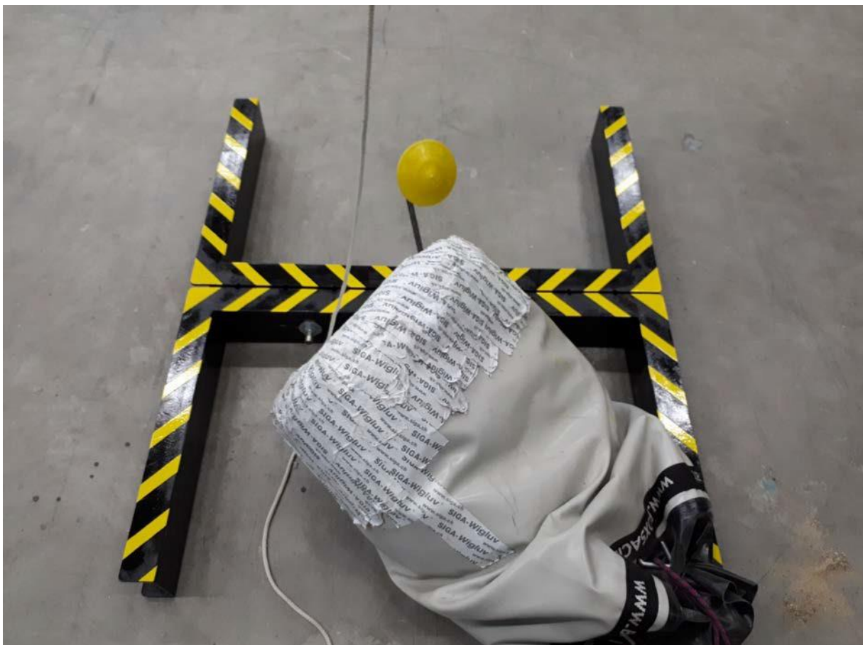
Figure 8: Situation after impact with a rod diameter d=12\text{mm} , buckling
