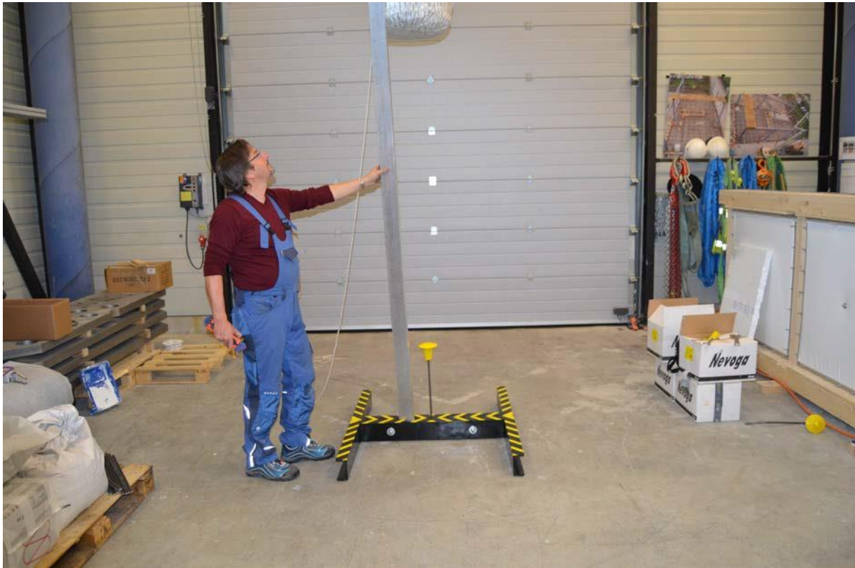
Figure 7: Lifting the fall sack and checking the fall height 3m for a rod diameter d=12\text{mm}
