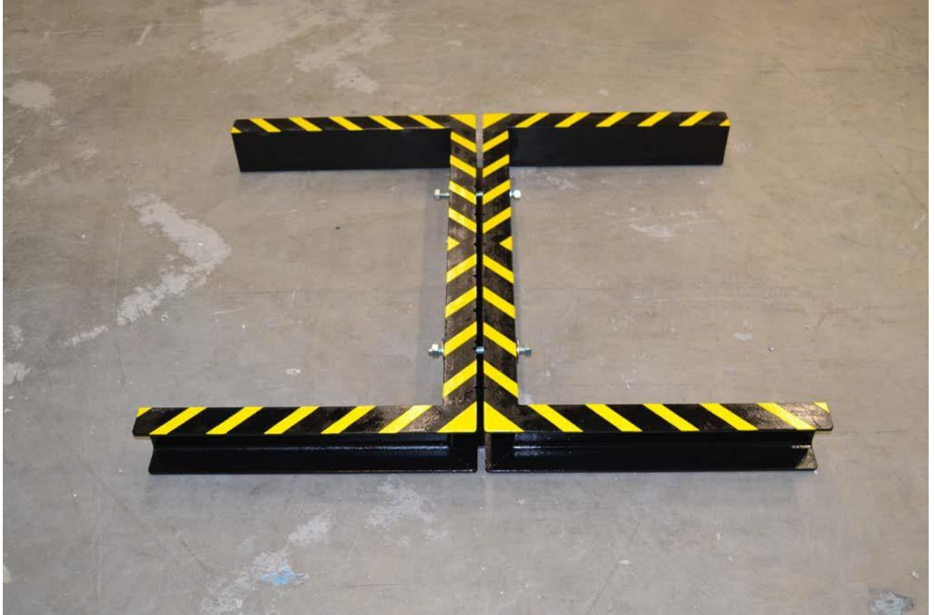
Figure 5: Mobile clamping frame made of construction steel
