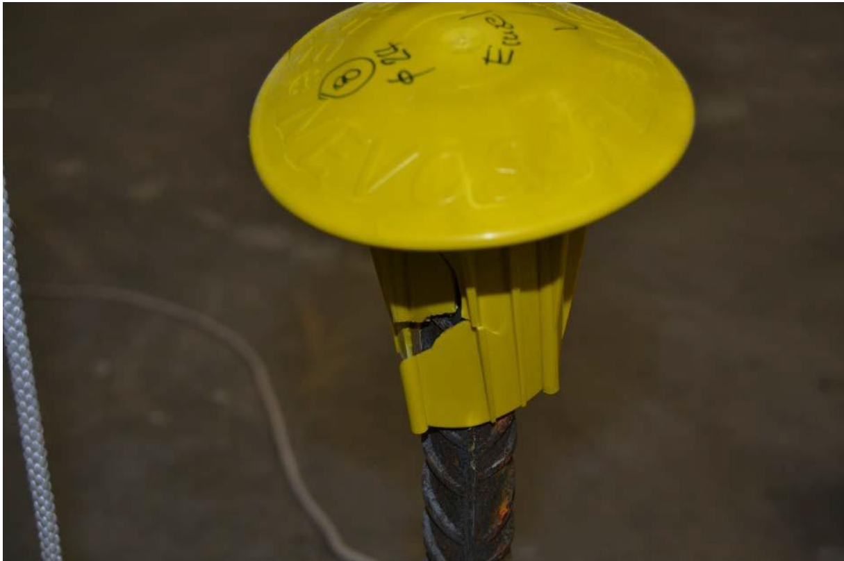
Figure 11: Test body 8 with deformation and slight twisting but without shear punching
